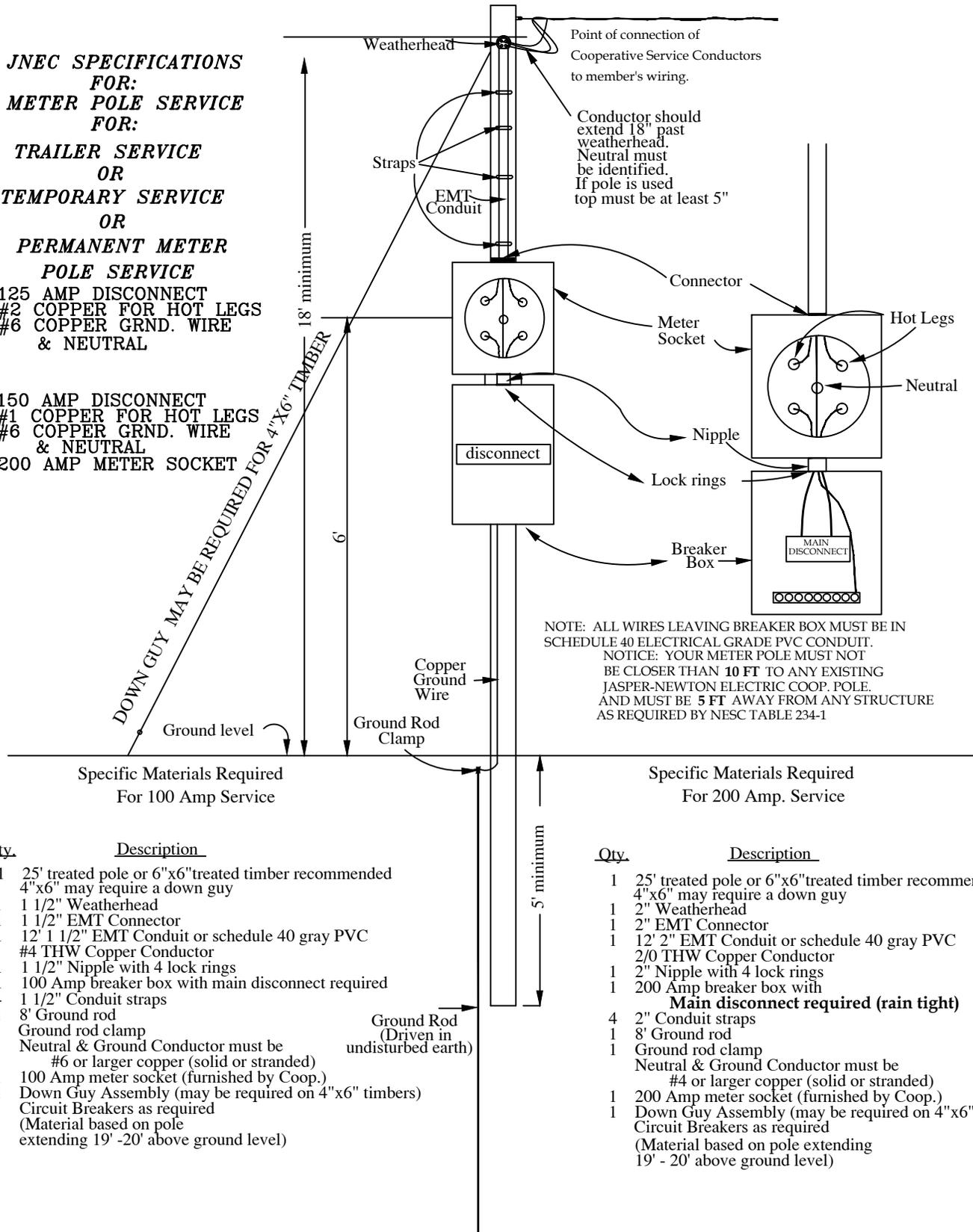
NOTE: ALL WIRES LEAVING BREAKER BOX MUST BE IN SCHEDULE 40 ELECTRICAL GRADE PVC CONDUIT.
